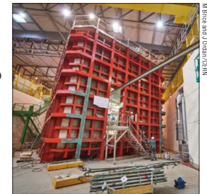
Prototype liquid-argon detectors for the international DUNE project are currently being built at CERN.
